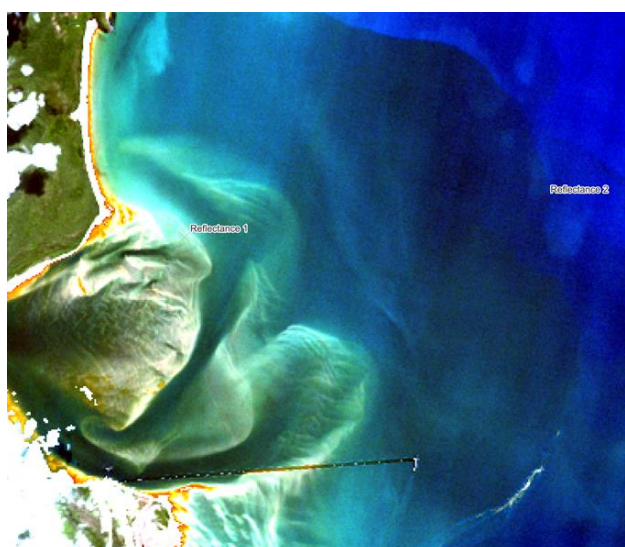
Figure 7-33 Water Leaving Reflectance of scene-ID 23601 for the AOI; Wavelengths for RGB: 611.02nm – 550.69nm – 463.73nm
